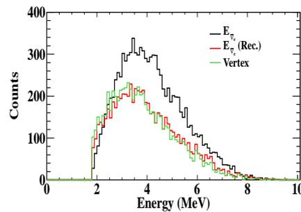
FIG. 1: Comparisons of reconstructed and input  $E_{\bar{\nu}_e}$  distribution, black line input energy, red line and green line show reconstructed and vertex energy of neutrino respectively
