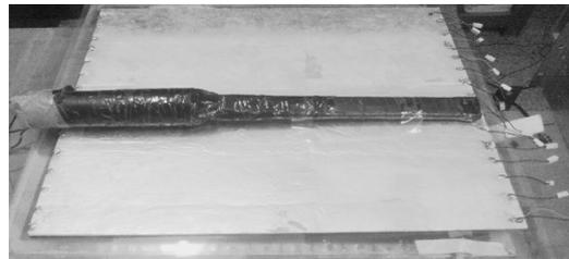
**Fig. 2:** Experimental arrangement for the efficiency measurement using finger type two plastic scintillator detectors.
