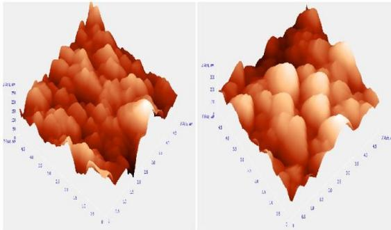
FIG. 3: 3-Dimensional atomic force microscopy (AFM) image of “as-deposited” (left panel) and “2 hours humid air exposed” (right panel) of KBr thin film photocathode.
