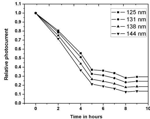
FIG. 1: Degradation in relative photocurrent as a function of time with humid air exposure on wavelengths 125 nm, 131 nm, 138 nm and 144 nm for 300 nm thick KBr film.
