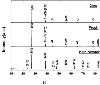
FIG. 2: XRD pattern of “as-deposited”, “2 hours humid air aged” 300 nm thick KBr film deposited on Al disc and of KBr powder.
