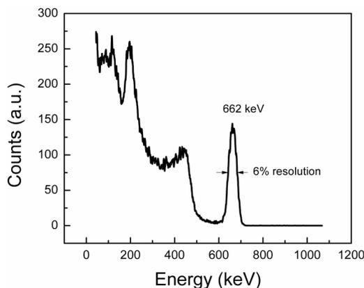
Fig.3: Pulse height spectrum of SrI<sub>2</sub>:Eu under <sup>137</sup>Cs gamma ray excitation
