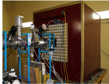
Fig.2. BRAHMMA subcritical core coupled to neutron generator
