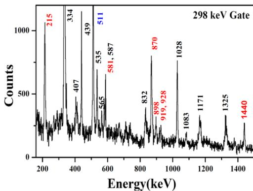
Figure 3: Gated spectrum of 298 keV. Peaks marked with red are the new transitions which have been confirmed to be present in  $^{150}\text{Sm}$ .
