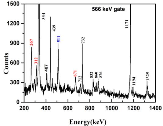
Figure 4: Gated spectrum of 566 keV. Peaks marked with red are the new transitions which have been confirmed to be present in  $^{150}\text{Sm}$ .
