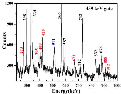
Figure 2: Gated spectrum of 439 keV. Peaks marked with red are the new transitions which have been confirmed to be present in  $^{150}\text{Sm}$ .
