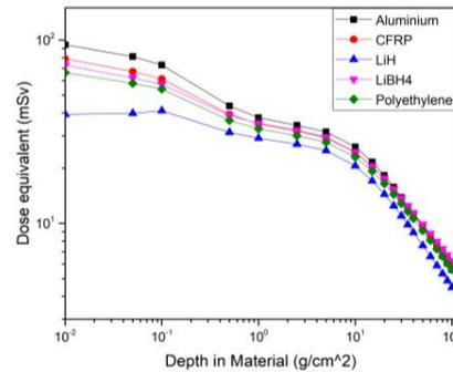
**Fig. 2.** Dose equivalent values at various depths inside water after 30 g/cm2 shielding materials for GCR environment.
