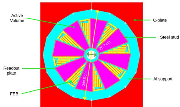
FIG. 1: Schematic of Improved Geometry of Station 1-Layer 1 (tag v211)
