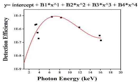
FIG. 4: Fitted efficiency curve for SDD.
