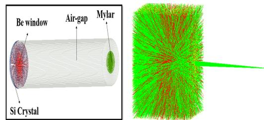
FIG. 2: (a) Simulated geometry of the SDD (b) Track structure produced by X-rays irradiating SDD.
