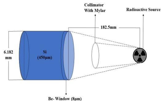
FIG. 1: Schematic diagram of the SDD.
