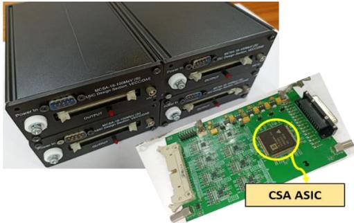
Fig. 2: MSCA-16 modules, PCB and CSA ASIC
