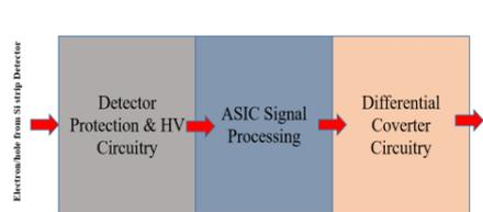
**Fig. 1:** Single channel block diagram of MCSA-16 Module
