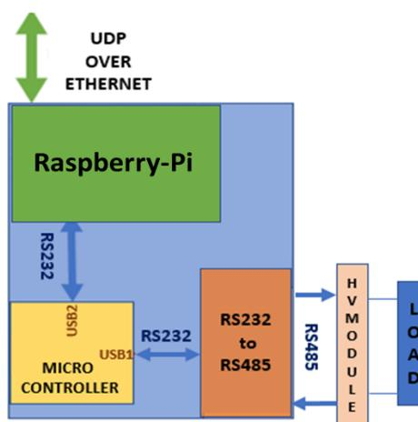
**Fig. 2** Block diagram of HV prototype supply
