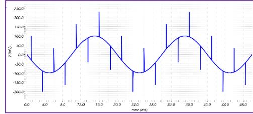
Fig. 3: CSA output without leakage current compensation circuit.
