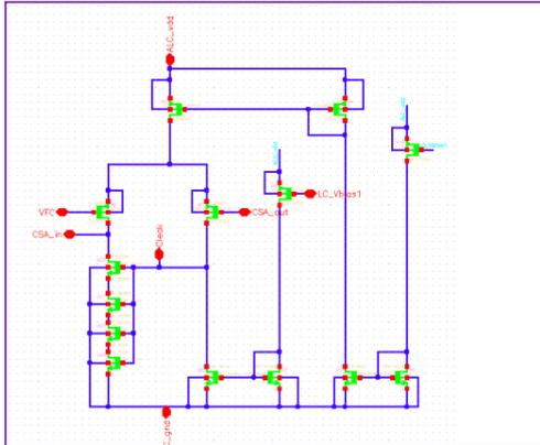
Fig. 2: CMOS implementation of LCC.
