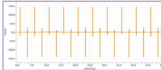
Fig. 4: CSA output without leakage current compensation circuit.
