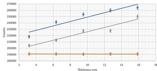
**Fig 4:** Area Under Backscattering Peak vs Thickness for different scattering materials (point source, experimental)
