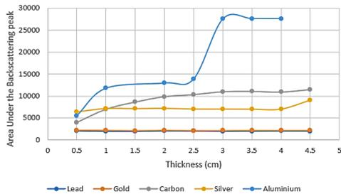
**Fig 3:** Area Under Backscattering Peak vs Thickness for different scattering materials (pencil beam emission source, simulated)
