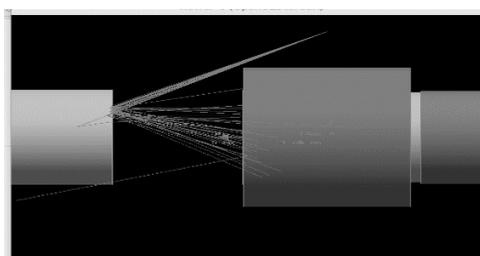
**Fig 1:** Detector Construction in Geant4, Detector (dark grey) and Scatterer (light grey) showing 50 events of point source under pencil beam emission {from visualization of the detector simulation through Open GUI}
