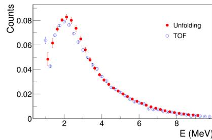
FIG. 2: Neutron energy spectrum obtained using PH unfolding and TOF method.
